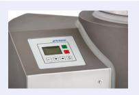
• The stand-alone deduster KD7010 and the KD7030 use the frequency converter KC7020 with LCD screen. The operator can turn the machine on and off, and chose the necessary conveying speed to operate with the tablet press
