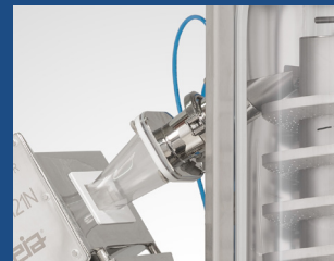
Dust-tight connection inclu- ding test tablet insert
