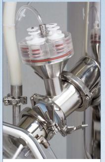
+ The tablet test sample dispenser KT2010 is an innovation that allows for easy contained metal detector sample tablet insertion without breaking containment
